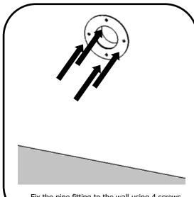
Fix the pipe fitting to the wall using 4 screws suitable to the wall type (countersunk screws)
