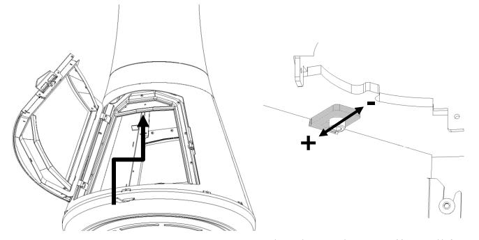
The top glass screen cleaning register(s) is accessible from inside the fireplace.
